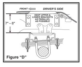
stack **see Figures "A" & "D"**. Fasten the bracket strap to the carriage bolts using two 3/8"- 16 flanged hex nuts. Note: F-450's & F-550's will clamp around the overload springs only, **see Figures "D" & "E"**. Slide the lower bracket forward or backward to align the air spring as close to vertical as possible. Tighten the 3/8" - 16 flanged hex bolt that holds the air spring to the lower bracket.
